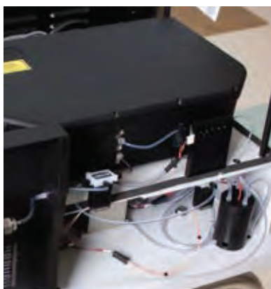
Hermetically sealed spectrometer eliminates frequent desiccant regeneration.
